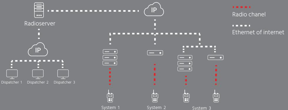
**ConSEL PLUS IS A SCALABLE SOLUTION,** compatible with MOTOTRBO equipment, allowing connection to one or more systems, thus ensuring the possibility of integration and communication between their users and dispatchers.
