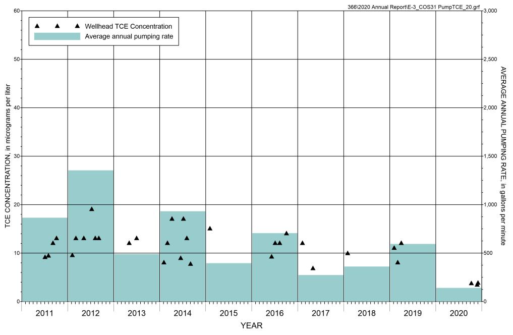
FIGURE E-3. CONCENTRATION OF TCE AND AVERAGE ANNUAL PUMPING RATE AT EXTRACTION WELL COS-31
