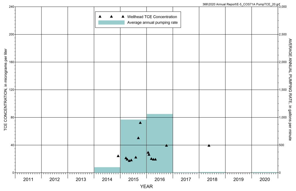
FIGURE E-5. CONCENTRATION OF TCE AND AVERAGE ANNUAL PUMPING RATE AT EXTRACTION WELL COS-71A
