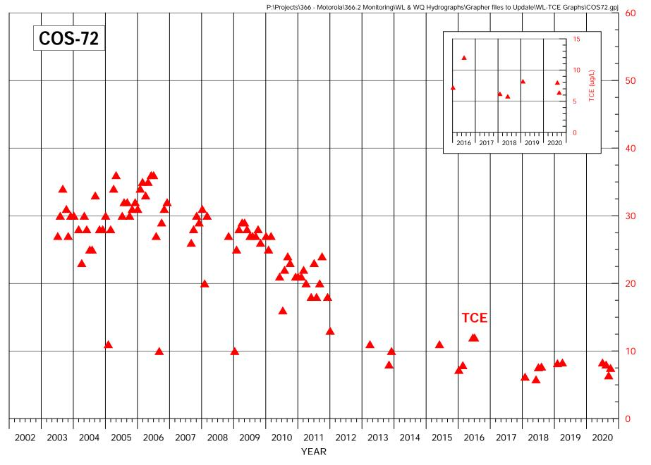
FIGURE D-6. TCE CONCENTRATIONS FOR EXTRACTION WELL COS-72
