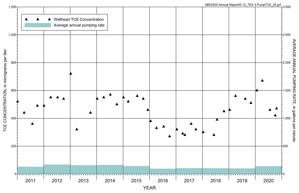
FIGURE E-12. CONCENTRATION OF TCE AND AVERAGE ANNUAL PUMPING RATE AT EXTRACTION WELL 7EX-3aMA 2011 THROUGH 2020
