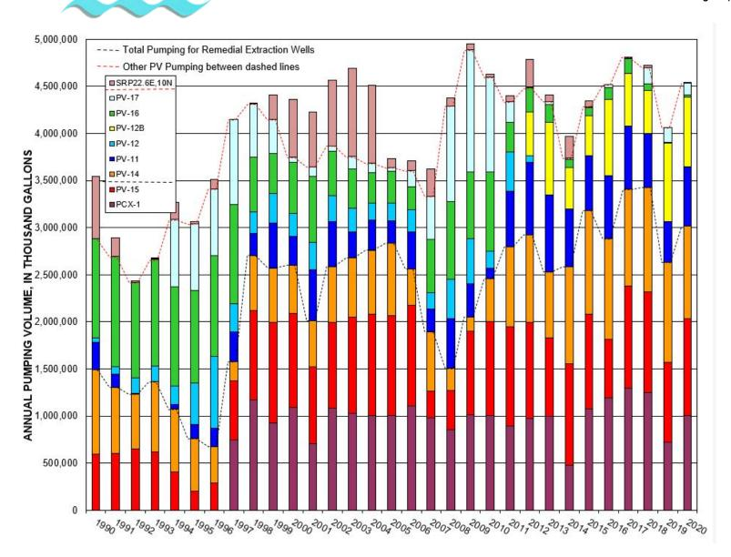
Figure 19. Distribution of Pumping in PV Wellfied
