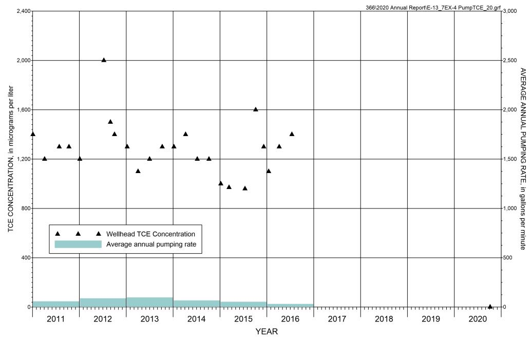
FIGURE E-13. CONCENTRATION OF TCE AND AVERAGE ANNUAL PUMPING RATE AT EXTRACTION WELL 7EX-4MA
