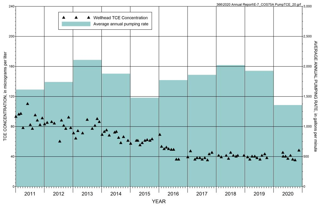
FIGURE E-7. CONCENTRATION OF TCE AND AVERAGE ANNUAL PUMPING RATE AT EXTRACTION WELL COS-75A 2011 THROUGH 2020
