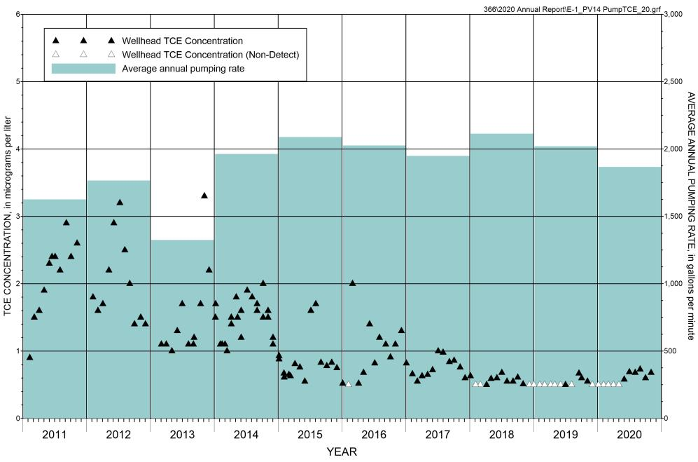
FIGURE E-1. CONCENTRATION OF TCE AND AVERAGE ANNUAL PUMPING RATE AT EXTRACTION WELL PV-14
