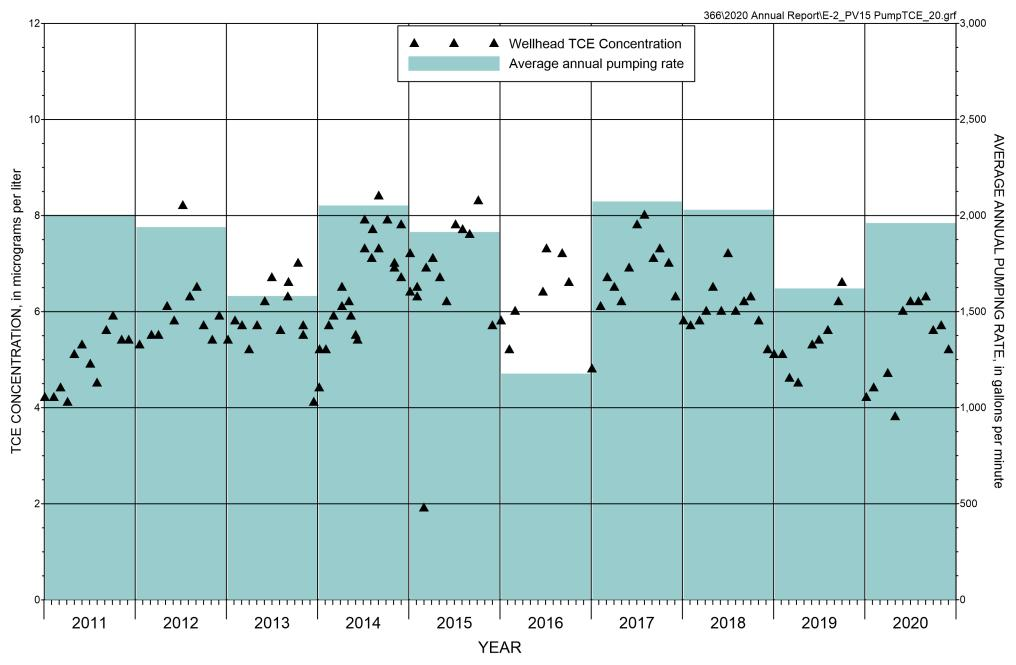
FIGURE E-2. CONCENTRATION OF TCE AND AVERAGE ANNUAL PUMPING RATE AT EXTRACTION WELL PV-15
