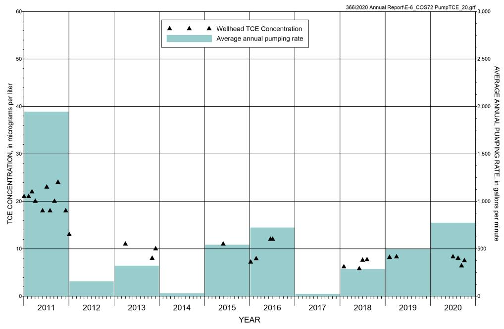
FIGURE E-6. CONCENTRATION OF TCE AND AVERAGE ANNUAL PUMPING RATE AT EXTRACTION WELL COS-72
