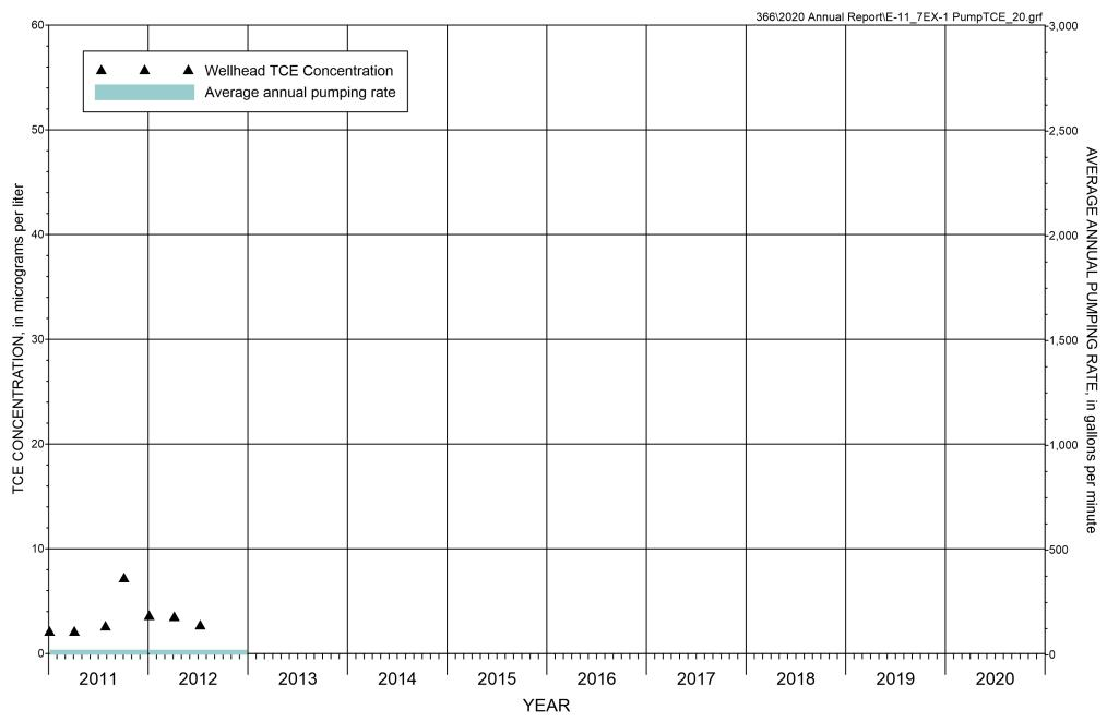
FIGURE E-11. CONCENTRATION OF TCE AND AVERAGE ANNUAL PUMPING RATE AT EXTRACTION WELL 7EX-1UA 2011 THROUGH 2020
