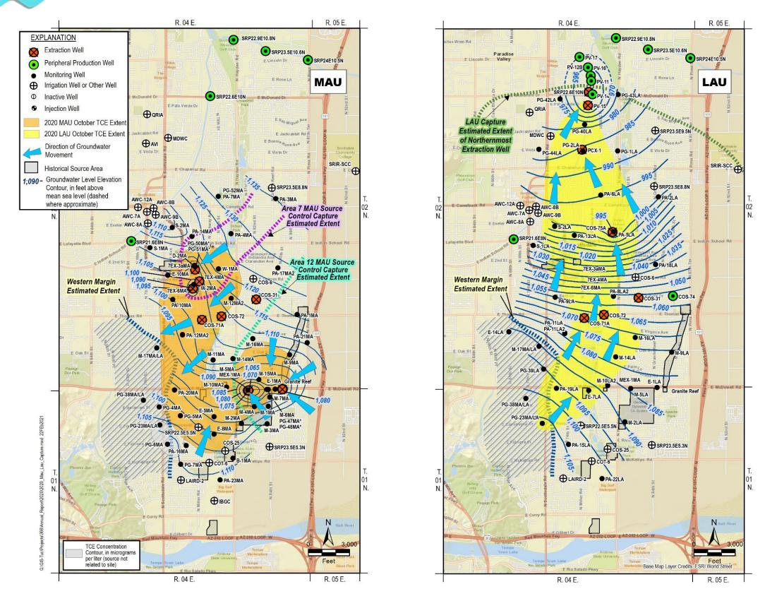
Figure 17. Estimated Hydraulic Capture of TCE Plume by MAU Source Control and Northernmost LAU Extraction Well for October 2020
