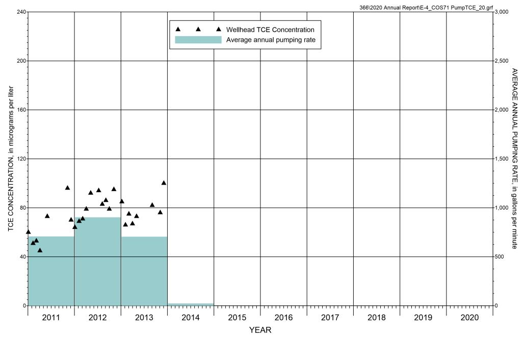
FIGURE E-4. CONCENTRATION OF TCE AND AVERAGE ANNUAL PUMPING RATE AT EXTRACTION WELL COS-71
