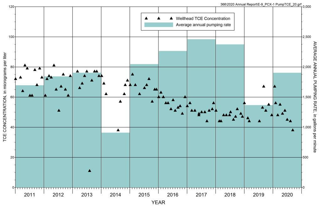
FIGURE E-9. CONCENTRATION OF TCE AND AVERAGE ANNUAL PUMPING RATE AT EXTRACTION WELL PCX-1 2011 THROUGH 2020 North Indian Bend Wash Superfund Site
