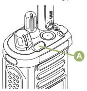
The Top Lightbar (A) indicates the secondary function of MFK and also the status of Intelligent Lighting.
