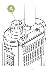
The Top Lightbar (A) indicates the secondary function of MFK and also the status of Intelligent Lighting.
