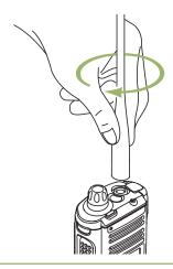
**3** To remove the antenna, turn the antenna counterclockwise.
