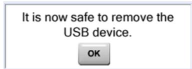
4. Touch **OK** and remove the USB thumb drive from the 4RE DVR.
